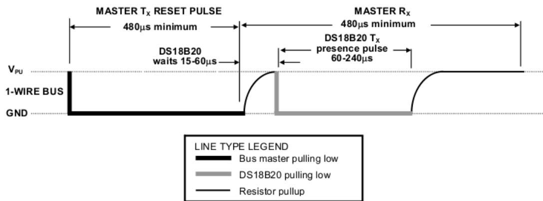
As you can see, in the reset pulse the master pulls the line low for a minimum of 480 µs and finally it releases the line. After that there is a period of 15-60µs to let the thermometer receive the rising edge (caused by the 4K7 resistor connected to VCC+) and emit the presence pulse, which is 60-240µs long. Just note that the second part (including the 15-60µs delay) must be 480µs long, too.
