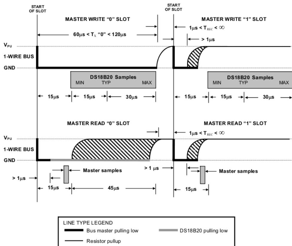
In the write operation, we always have to pull the line low at startup. If we want to write 0 we
